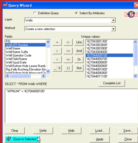
Above: The Query Wizard dialog box displaying a Select By Attributes query to select Well API Number = 427044000100.
